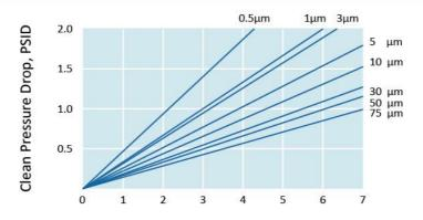
Flow Rate, GPM, Water@AMB.
