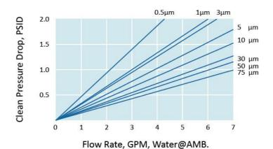
Flow rate is per 10" cartridge. For liquids other than water, multiply the pressure drop by the fluid viscosity in centipoises
